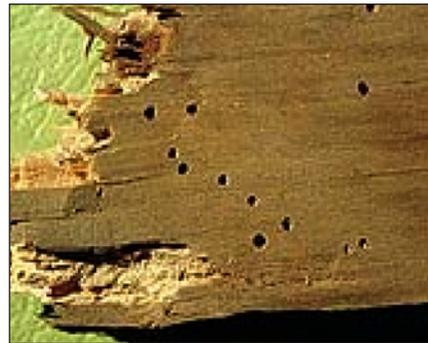
Figure 5. Wood damaged by powderpost beetles.
