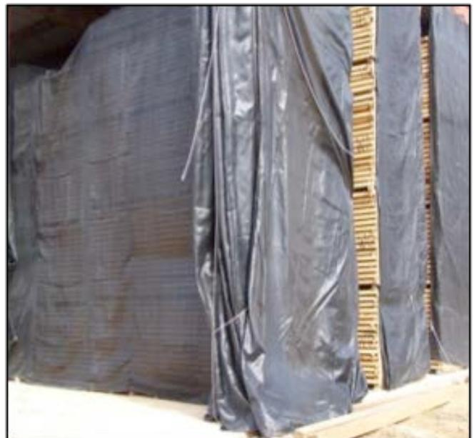
Figure 4. Dry-end storage using a T-shed and mesh covered stacks (photos courtesy of Dr. Kevin Ragon, Quality Pole Inspection and Maintenance, Inc.).
