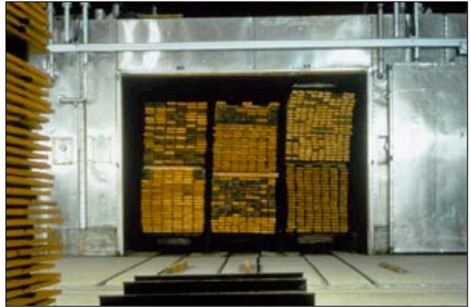
Figure 2. An industrial-scale kiln can dry large volumes of hardwood lumber.
